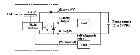
\*Self-diagnosis output self-diagnosis output is continued to execute(ON) and when light-entering level would be kept in +/-15% range of operation level(ON and OFF point) for 0.3sec or more, this output would be getting OFF. If necessary, cut this cable(Yellow/red) at the Base.
